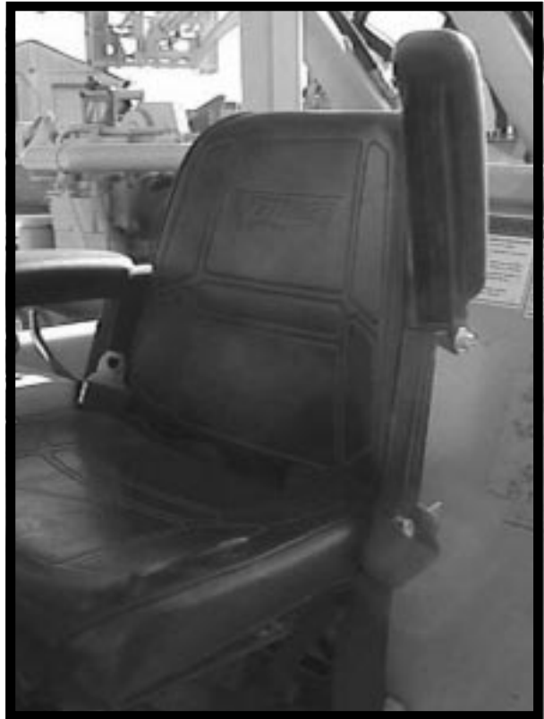
Fig. 2-1, Arm rest shown in the up position for entering and exiting the operator's compartment.
